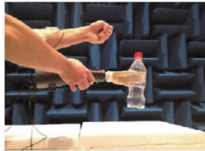
Fig.2 Myoelectric artificial hand system for emission measurement
